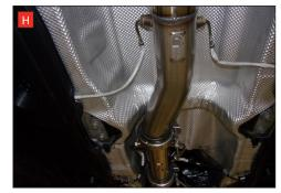
G) Re-fit the heat sheild wrap over the hoses and re-fit the propshaft heat sheild.
